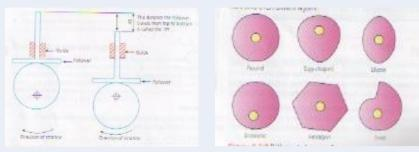
The pattern of movement is determined by the design / shape of the cam, i.e. if the cam is round with the shaft in the centre the follower will remain stationary, however if the cam is round but the shaft is off centre then the follower will continually rise and fall. There are many shapes of cams:
